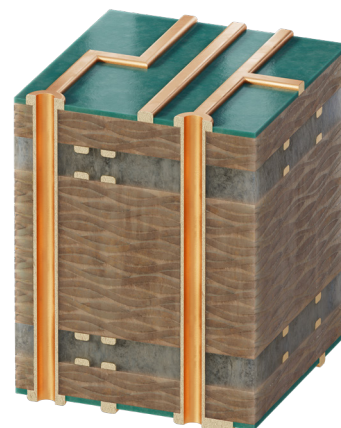
Figure 1. SFL-12 PCB stackup
