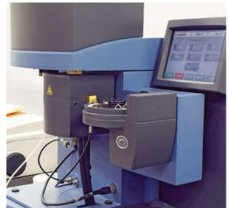
Thermogravimetric Analyzer (TGA) – Measures the stability of our dielectrics at high temperatures, baking the materials at prescribed temperatures and measuring weight loss.
