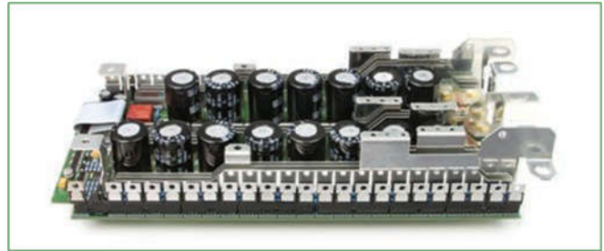
(66) Thru-hole FETs (15) High profile capacitors (9) High profile bus bars Total Weight 3.4lbs (1543.6 g)
