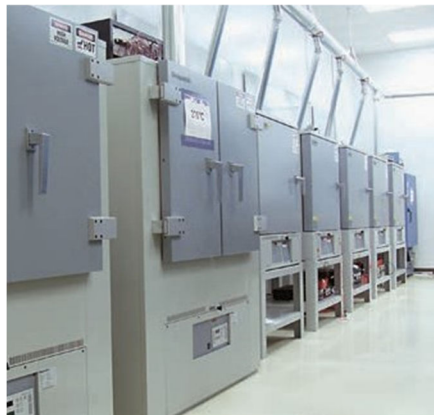
Chamber Ovens – dedicated to long term thermal bias age testing. The ovens take material to temperatures above Tg. At selected intervals, samples are removed and tested to verify material integrity.
