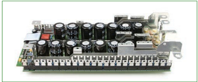
(66) Thru-hole FETs (15) High profile capacitors (9) High profile bus bars Total Weight 3.4lbs (1543.6 g)
