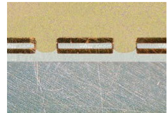
Laminated thick copper up to 5 oz. (175µm) finished on the internal layer using HT dielectric
